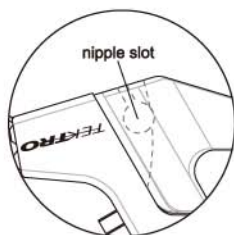
Lever showing single upper nipple slot
